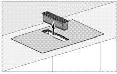
The oil filter may collect oil or overflowing liquids on its bottom surface. While the filter is being disassembled, it should be removed straight to prevent dripping and spilling.
