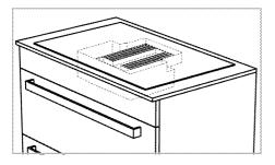
4. First of all, in order to remove one of the carbon filters from its magnetic slot from the ventilation gap, pull it towards you by tilting it and take it out as shown in the figure.
